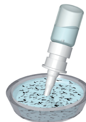
TSIT (Tip Seal Integrity Test)
