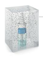
CVIT (Closure Ventilation Integrity Test) Closure and filter challenge with Bacillus atrophaeus spores
