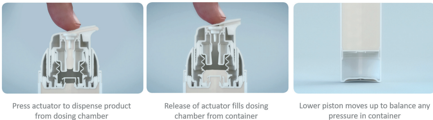
Figure 1: The principles of Airless piston technology.
