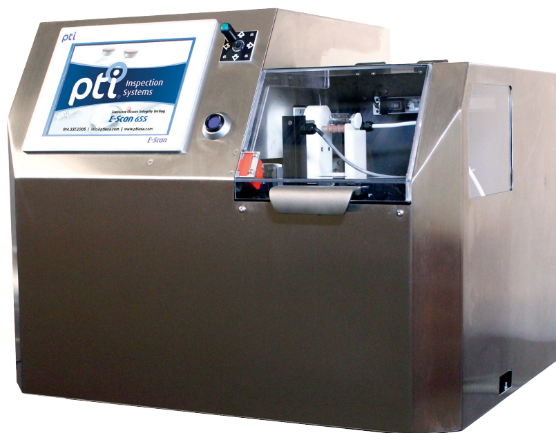
Figure 2: Example of HVLD equipment at Gateway Analytical.
